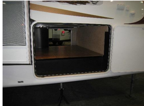
Basement Area/Pass Through Storage
